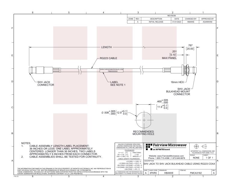
SHV Jack to SHV Jack Bulkhead Cable RG223 Coax in 24 Inch
