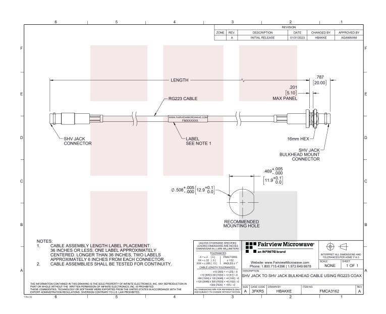
SHV Jack to SHV Jack Bulkhead Cable RG223 Coax in 48 Inch
