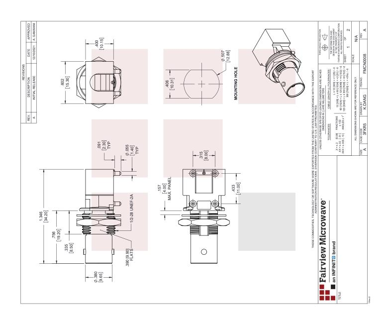
RA 75 Ohm 12G SDI BNC Female Bulkhead PCB Connector 0.062" Board Thickness Solder Attachment
