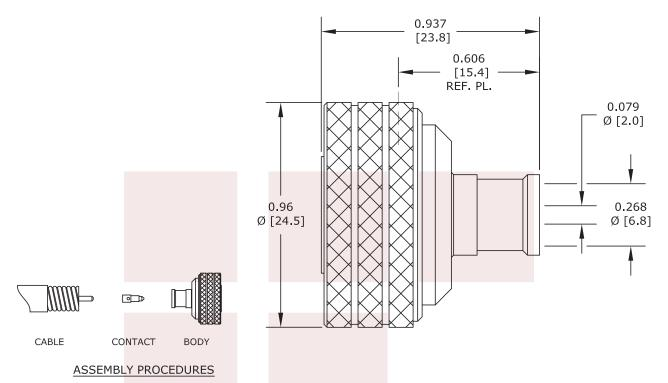
1. STRIP CABLE AS SHOWN, CHAMFER CENTER CONDUCTOR & DEBURR CABLE.
