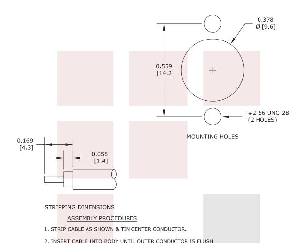
3. SOLDER OUTER CONDUCTOR TO BODY. PRESS DOWN CAP.
