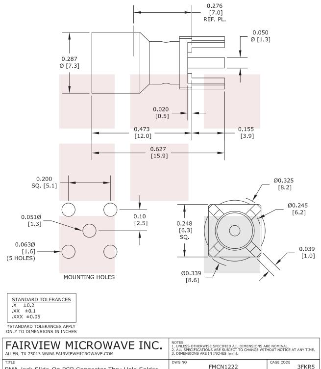
BMA Jack Slide-On PCB Connector Thru Hole Solder Attachment
