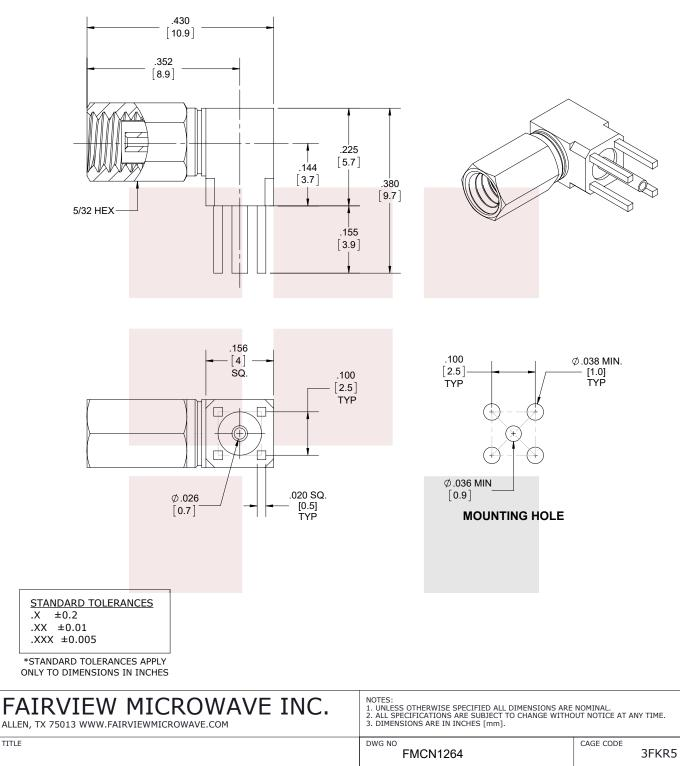
RA SSMC Plug PCB Connector Thru Hole Solder Attachment
