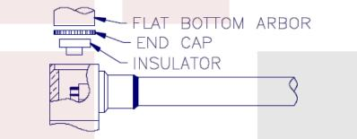
5. PRESS INSULATOR AND END CAP INTO CONNECTOR BODY AND USE A FLAT BOTTOM ARBOR TO PRESS CAP IN PLACE. CAP MUST BE BELOW BODY SURFACE TO SEAT PROPERLY.
