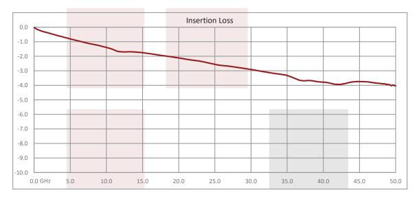
Measurement is for two connectors with 1.0 inch (25.4mm) length of substrate
