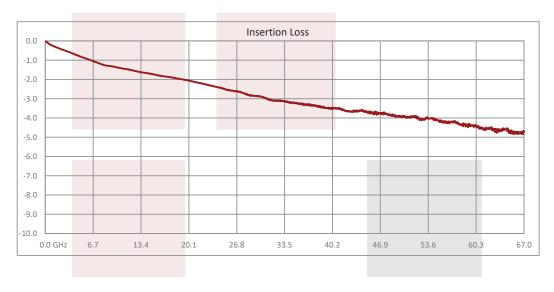
Measurement is for two connectors with 1.0 inch (25.4mm) length of substrate
