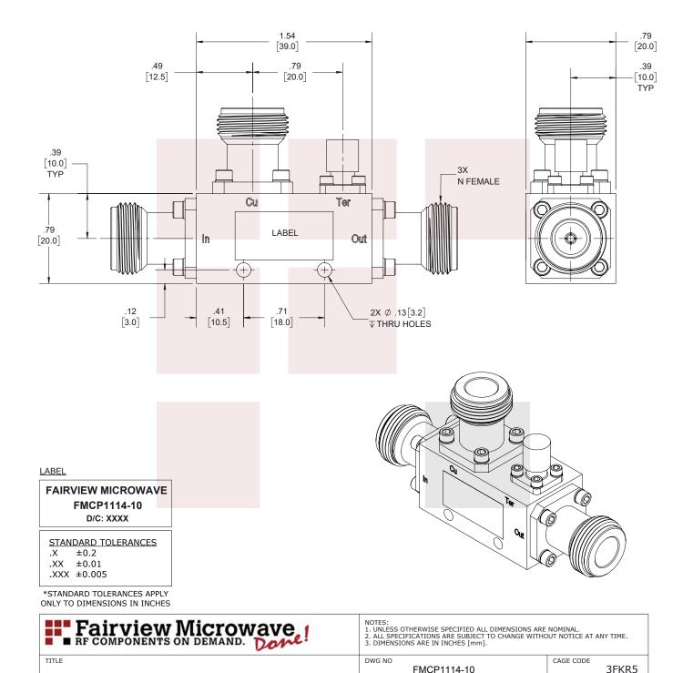
N Directional Coupler 10 dB 4 GHz to 18 GHz Rated to
