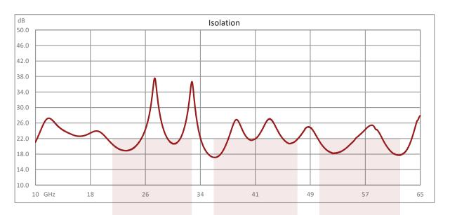
2 Way Power Divider 1.85mm Interface from 10 GHz to 65 GHz Rated at 10 Watts from Fairview Microwave is in-stock and available to ship same-day. All of our RF/microwave products are available off-the-shelf from our ISO 9001:2008 certified facilities in Lewisville, Texas. Fairview Microwave is RF on-demand.
