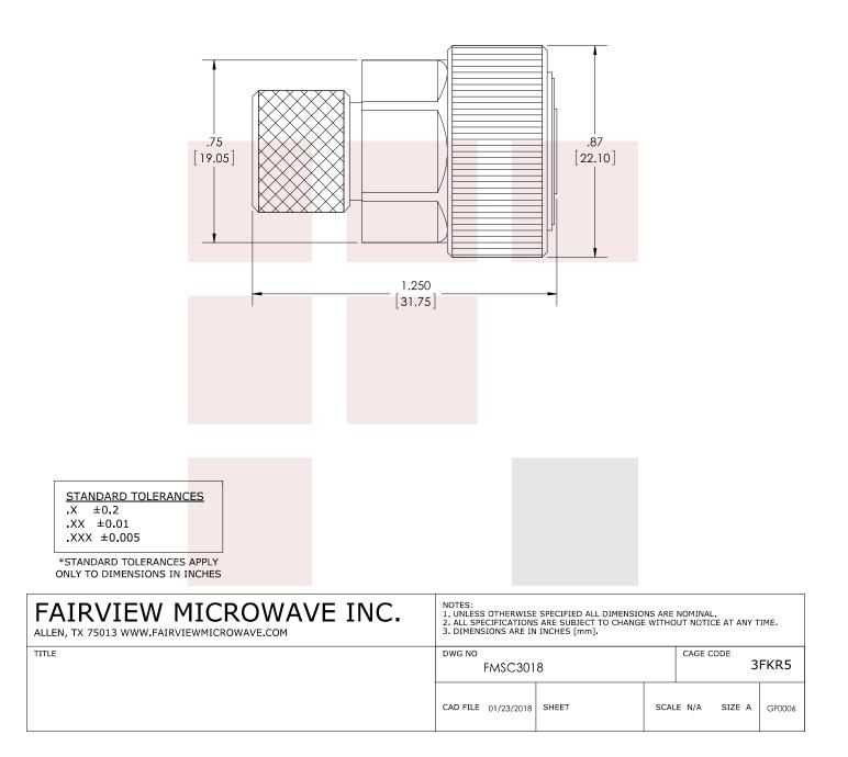
7mm Short Calibration Kit Component for Precision Up to 18  $\mbox{GHz}$
