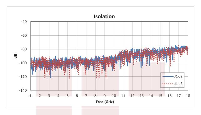
SMA PIN Diode Switch SPDT From 1 GHz to 18 GHz Rated at +20 dBm from Fairview Microwave is in-stock and available to ship same-day. All of our RF/microwave products are available off-the-shelf from our ISO 9001:2008 certified facilities in Allen, Texas. Fairview Microwave is RF on-demand.
