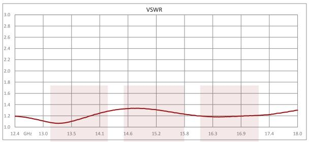
WR-62 to SMA Female Waveguide to Coax Adapter UG-1665/U Square Cover Flange With 12.4 GHz to 18 GHz Frequency Range For Ku Band from Fairview Microwave is in-stock and available to ship same-day. All of our RF/microwave products are available off-the-shelf from our ISO 9001:2008 certified facilities in Allen, Texas. Fairview Microwave is RF on-demand.
