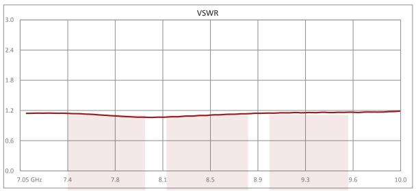
WR-112 to N Female Waveguide to Coax Adapter UG-51/U Square Cover Flange With 7.05 GHz to 10 GHz Frequency Range For H Band from Fairview Microwave is in-stock and available to ship same-day. All of our RF/microwave products are available off-the-shelf from our ISO 9001:2008 certified facilities in Allen, Texas. Fairview Microwave is RF on-demand.
