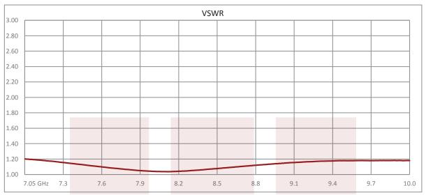
WR-112 to SMA Female Waveguide to Coax Adapter CPR-112G Grooved with 7.05 GHz to 10 GHz H Band in Aluminum, Paint from Fairview Microwave is in-stock and available to ship same-day. All of our RF/microwave products are available off-the-shelf from our ISO 9001:2008 certified facilities in Allen, Texas. Fairview Microwave is RF on-demand.
