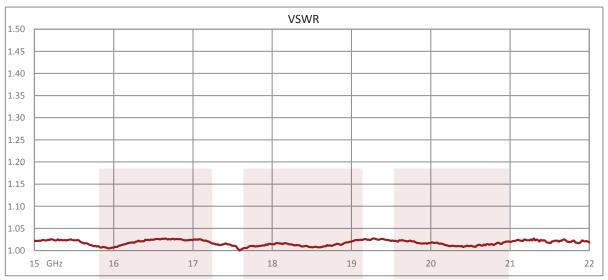
Commercial Grade WR-51 Waveguide Termination 1 Watt With a 15 GHz to 22 GHz Frequency Range from Fairview Microwave is in-stock and available to ship same-day. All of our RF/microwave products are available off-the-shelf from our ISO 9001:2008 certified facilities in Allen, Texas. Fairview Microwave is RF on-demand.
