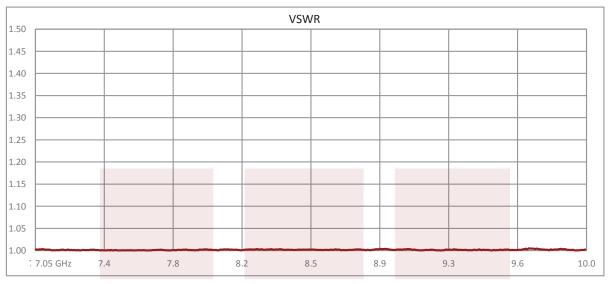
Commercial Grade WR-112 Waveguide Termination 5 Watts With a 7.05 GHz to 10 GHz Frequency Range from Fairview Microwave is in-stock and available to ship same-day. All of our RF/microwave products are available off-the-shelf from our ISO 9001:2008 certified facilities in Allen, Texas. Fairview Microwave is RF on-demand.
