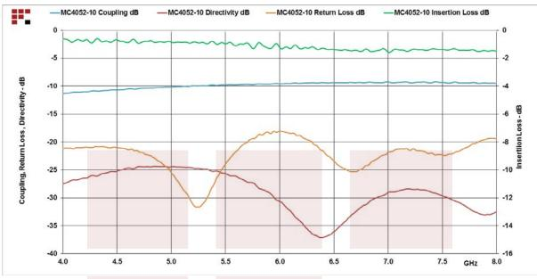
N Directional Coupler 10 dB Coupled Port From 4 GHz to 8 GHz Rated To 50 Watts from Fairview Microwave is in-stock and available to ship same-day. All of our RF/microwave products are available off-the-shelf from our ISO 9001:2008 certified facilities in Allen, Texas. Fairview Microwave is RF on-demand.
