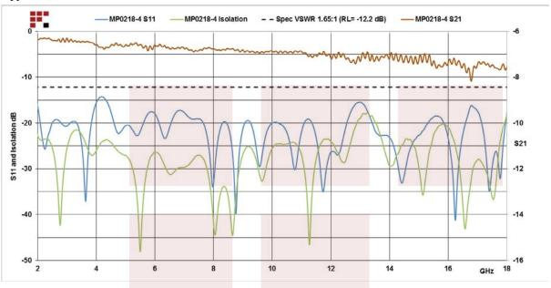
4 Way Power Divider SMA Connectors From 2 GHz to 18 GHz Rated at 30 Watts from Fairview Microwave is in-stock and available to ship same-day. All of our RF/microwave products are available off-the-shelf from our ISO 9001:2008 certified facilities in Allen, Texas. Fairview Microwave is RF on-demand.
