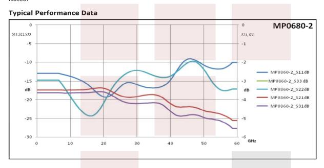
2 Way Power Divider 1.85mm Connectors From 8 GHz to 60 GHz Rated at 10 Watts from Fairview Microwave is in-stock and available to ship same-day. All of our RF/microwave products are available off-the-shelf from our ISO 9001:2008 certified facilities in Allen, Texas. Fairview Microwave is RF on-demand.
