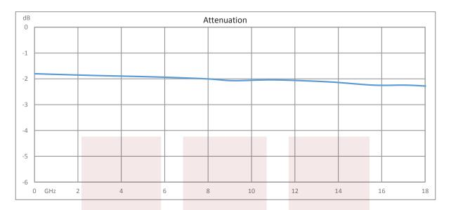
2 dB Fixed Attenuator SMA Male To SMA Female Up To 18 GHz Rated To 2 Watts With Passivated Stainless Steel Body from Fairview Microwave is in-stock and available to ship same-day. All of our RF/microwave products are available off-the-shelf from our ISO 9001:2008 certified facilities in Allen, Texas. Fairview Microwave is RF on-demand.
