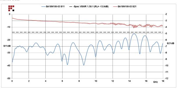
3 dB Fixed Attenuator N Male (Plug) to N Female (Jack) Up to 18 GHz Rated to 100 Watts, Heatsink Body, 1.45 VSWR from Fairview Microwave is in-stock and available to ship same-day. All of our RF/microwave products are available off-the-shelf from our ISO 9001:2008 certified facilities in Lewisville, Texas. Fairview Microwave is RF on-demand.
