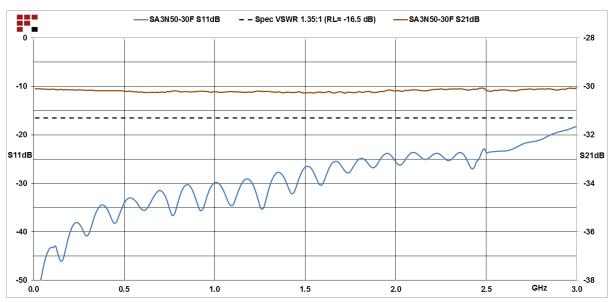
30 dB Fixed Attenuator N Female (Jack) to N Female (Jack) Up to 3 GHz Rated to 50 Watts, Heatsink Body, 1.35 VSWR from Fairview Microwave is in-stock and available to ship same-day. All of our RF/microwave products are available off-the-shelf from our ISO 9001:2008 certified facilities in Lewisville, Texas. Fairview Microwave is RF on-demand.
