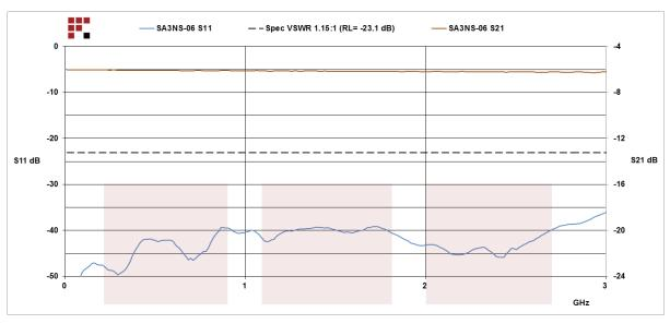
6 dB Fixed Attenuator N Male To N Female Up To 3 GHz Rated To 2 Watts With Brass Tri-Metal Body from Fairview Microwave is in-stock and available to ship same-day. All of our RF/microwave products are available off-the-shelf from our ISO 9001:2008 certified facilities in Allen, Texas. Fairview Microwave is RF on-demand.
