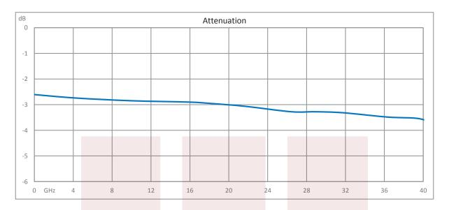
3 dB Fixed Attenuator 2.92mm Male To 2.92mm Female Up To 40 GHz Rated To 0.5 Watts With Passivated Stainless Steel Body from Fairview Microwave is in-stock and available to ship same-day. All of our RF/microwave products are available off-the-shelf from our ISO 9001:2008 certified facilities in Allen, Texas. Fairview Microwave is RF on-demand.
