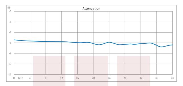
8 dB Fixed Attenuator 2.92mm Male To 2.92mm Female Up To 40 GHz Rated To 0.5 Watts With Passivated Stainless Steel Body from Fairview Microwave is in-stock and available to ship same-day. All of our RF/microwave products are available off-the-shelf from our ISO 9001:2008 certified facilities in Allen, Texas. Fairview Microwave is RF on-demand.
