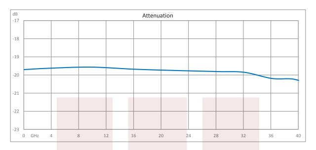
20 dB Fixed Attenuator 2.92mm Male To 2.92mm Female Up To 40 GHz Rated To 0.5 Watts With Passivated Stainless Steel Body from Fairview Microwave is in-stock and available to ship same-day. All of our RF/microwave products are available off-the-shelf from our ISO 9001:2008 certified facilities in Allen, Texas. Fairview Microwave is RF on-demand.
