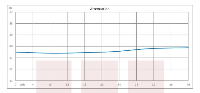
30 dB Fixed Attenuator 2.92mm Male To 2.92mm Female Up To 40 GHz Rated To 0.5 Watts With Passivated Stainless Steel Body from Fairview Microwave is in-stock and available to ship same-day. All of our RF/microwave products are available off-the-shelf from our ISO 9001:2008 certified facilities in Allen, Texas. Fairview Microwave is RF on-demand.
