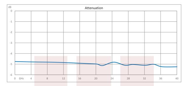
5 dB Fixed Attenuator 2.92mm Male To 2.92mm Female Up To 40 GHz Rated To 1 Watt With Passivated Stainless Steel Body from Fairview Microwave is in-stock and available to ship same-day. All of our RF/microwave products are available off-the-shelf from our ISO 9001:2008 certified facilities in Allen, Texas. Fairview Microwave is RF on-demand.
