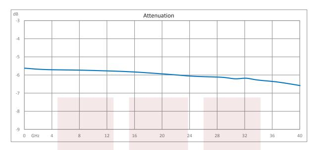
6 dB Fixed Attenuator 2.92mm Male To 2.92mm Female Up To 40 GHz Rated To 1 Watt With Passivated Stainless Steel Body from Fairview Microwave is in-stock and available to ship same-day. All of our RF/microwave products are available off-the-shelf from our ISO 9001:2008 certified facilities in Allen, Texas. Fairview Microwave is RF on-demand.
