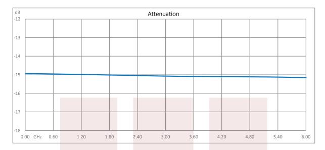
15 dB Fixed Attenuator QMA Male To QMA Female Up To 6 GHz Rated To 2 Watts With Brass Tri-Metal Body from Fairview Microwave is in-stock and available to ship same-day. All of our RF/microwave products are available off-the-shelf from our ISO 9001:2008 certified facilities in Allen, Texas. Fairview Microwave is RF on-demand.
