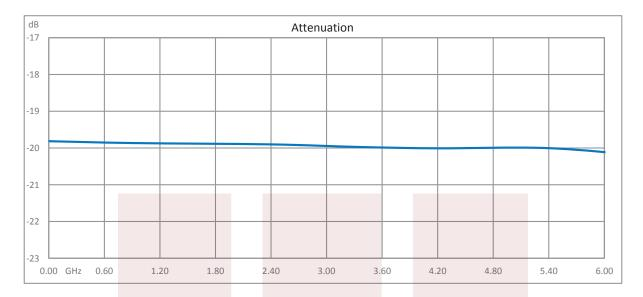
20 dB Fixed Attenuator QMA Male To QMA Female Up To 6 GHz Rated To 2 Watts With Brass Tri-Metal Body from Fairview Microwave is in-stock and available to ship same-day. All of our RF/microwave products are available off-the-shelf from our ISO 9001:2008 certified facilities in Allen, Texas. Fairview Microwave is RF on-demand.
