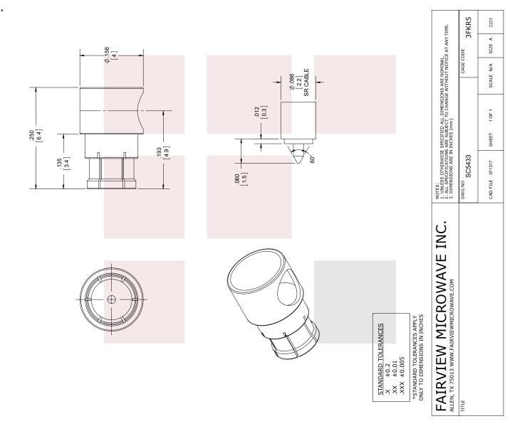
RA Mini SMP Female Connector Solder Attachment For RG405 Cable
