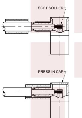
2.) INSTALL CABLE INTO BODY ASSEMBLY SO THE TUBE PORTION OF THE BODY SLIDES UNDER THE CABLE BRAID. PUSH CABLE FORWARD UNTIL CENTER CONDUCTOR IS IN SLOT OF CONTACT AND CABLE BRAID MEETS CONNECTOR BODY. SOFT SOLDER CENTER CONDUCTOR IN PLACE.
