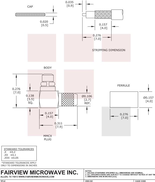
TILE RA MMCX Plug Connector Crimp/Solder Attachment For 0.100 inch, RG316, RG174, RG188, LMR-100, LMR-100A, LMR-100A-FR Cable
