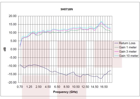
Gain Horn Antenna Operating From 700 MHz to 18 GHz With a Nominal 10 dBi Typical Gain With N Female Input Connector from Fairview Microwave is in-stock and available to ship same-day. All of our RF/microwave products are available off-the-shelf from our ISO 9001:2008 certified facilities in Lewisville, Texas. Fairview Microwave is RF on-demand.
