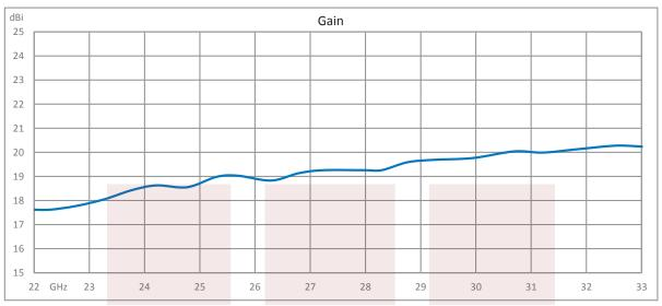
WR-34 Standard Waveguide Horn With Square Cover Flange and 20 dBi Nominal Gain Operating From 22 GHz to 33 GHz Frequency Range from Fairview Microwave is in-stock and available to ship same-day. All of our RF/microwave products are available off-the-shelf from our ISO 9001:2008 certified facilities in Allen, Texas. Fairview Microwave is RF on-demand.
