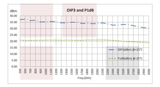
2.6 dB NF Low Noise Amplifier Operating From 500 MHz to 3 GHz with 29 dB Gain, 20 dBm P1dB and SMA from Fairview Microwave is in-stock and available to ship same-day. All of our RF/microwave products are available off-the-shelf from our ISO 9001:2008 certified facilities in Allen, Texas. Fairview Microwave is RF on-demand.
