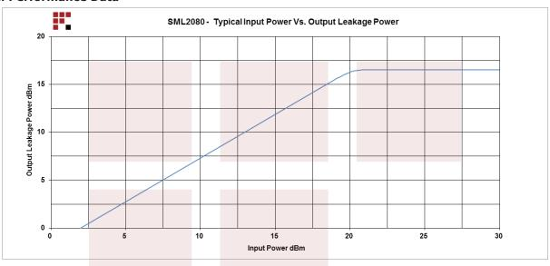
SMA Limiter PIN-Schottky With 16 dBm Flat Leakage Operating From 2 GHz to 8 GHz from Fairview Microwave is in-stock and available to ship same-day. All of our RF/microwave products are available off-the-shelf from our ISO 9001:2008 certified facilities in Allen, Texas. Fairview Microwave is RF on-demand.
