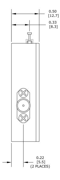
NOTE: HEAT SINK REQUIRED FOR PROPER OPERATION, UNIT IS COOLED BY CONDUCTING TO HEAT SINK.
