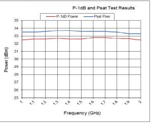
Medium Power Amplifier at 2 Watt P1dB Operating From 1 GHz to 2 GHz with 35 dB Gain, 45 dBm IP3 and SMA from Fairview Microwave is in-stock and available to ship same-day. All of our RF/microwave products are available off-the-shelf from our ISO 9001:2008 certified facilities in Lewisville, Texas. Fairview Microwave is RF on-demand.
