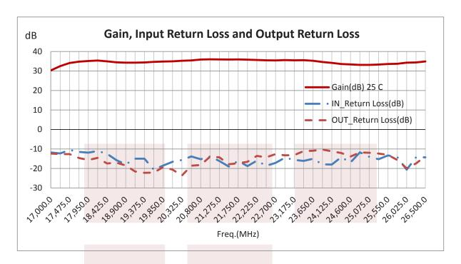
Medium Power GaAs Amplifier at 1 Watt P1dB Operating from 18 GHz to 26.5 GHz with 38 dBm IP3, 2.92mm Input, 2.92mm Output and 33 dB Gain from Fairview Microwave is in-stock and available to ship same-day. All of our RF/microwave products are available off-the-shelf from our ISO 9001:2008 certified facilities in Allen, Texas. Fairview Microwave is RF on-demand.
