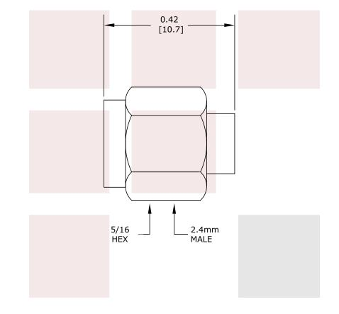
$\begin{array}{l} \text{STANDARD TOLERANCES} \\ .X \quad \pm 0.2 \\ .XX \quad \pm 0.01 \\ .XXX \quad \pm 0.005 \end{array}$
