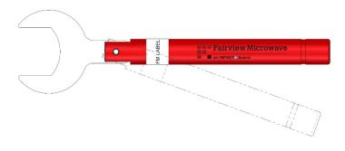
Torque wrench handle will break over when preset torque is achieved. Take note of the wrench bit orientation relative to the direction of motion/rotation.
