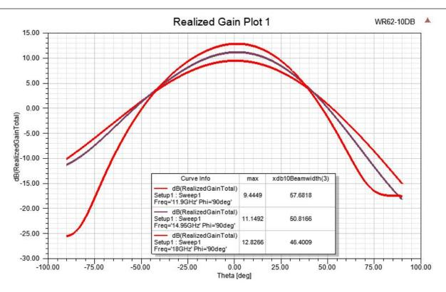
WR-62 Waveguide Antenna With 10 dBi Gain and 12.4 GHz to 18 GHz, Integrated Cage-Style Mount from Fairview Microwave is in-stock and available to ship same-day. All of our RF/microwave products are available off-the-shelf from our ISO 9001:2008 certified facilities in Lewisville, Texas. Fairview Microwave is RF on-demand.
