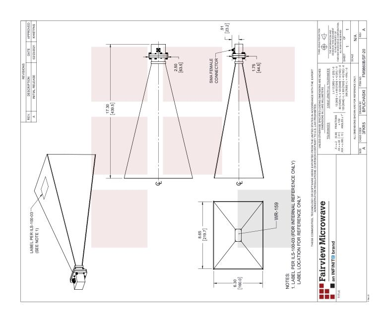
WR-159 Standard Gain Horn Antenna Operating From 4.9 GHz to 7.05 GHz, 20 dBi Nominal Gain, SMA Female Input Connector, ProLine
