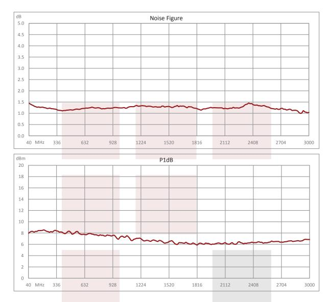
1.3 dB NF Low Noise Amplifier, Operating from 40 MHz to 3 GHz with 16 dB Gain, 7 dBm P1dB and SMA from Fairview Microwave is in-stock and available to ship same-day. All of our RF/microwave products are available off-the-shelf from our ISO 9001:2008 certified facilities in Lewisville, Texas. Fairview Microwave is RF on-demand.
