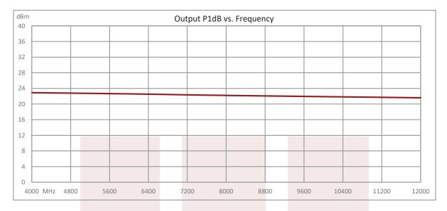
35 dB min Gain, Temperature Compensated Low Noise Amplifier, 22 dBm P1dB Operating from 4 GHz to 12 GHz with SMA from Fairview Microwave is in-stock and available to ship same-day. All of our RF/microwave products are available off-the-shelf from our ISO 9001:2008 certified facilities in Lewisville, Texas. Fairview Microwave is RF on-demand.
