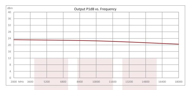
35 dB min Gain, Temperature Compensated Low Noise Amplifier, 22 dBm P1dB Operating from 2 GHz to 18 GHz with SMA from Fairview Microwave is in-stock and available to ship same-day. All of our RF/microwave products are available off-the-shelf from our ISO 9001:2008 certified facilities in Lewisville, Texas. Fairview Microwave is RF on-demand.
